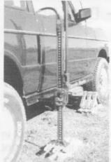
One of each pair of ChockTraks incorporates a cut out in the ground blades and side guides in which the base of a standard Hi-lift jack can nestle so reducing the chance of the jack sinking or slipping sideways because in the increased area of contact with the ground.
